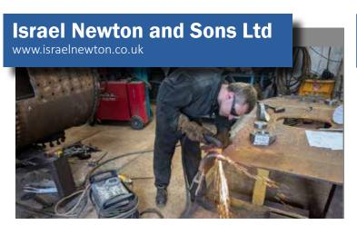
The business, run by two brothers, undertakes work on historic steam railway locomotive boilers and associated specialist engineering work. They undertake a complete service – from the smallest repair to the design, manufacture and assembly of an entire steam boiler.
